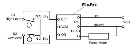
**Refill**: Low level permits S2 to close, starting refill pump. Rising level allows S2 to open and eventually closes S1 to actuate the FLIP-PAK "OFF" circuit and stop the pump motor. The FLIP-PAK "OFF" override assures pump shut-down even if S2 failed to open.
