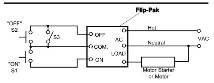
With two normally open momentary contact push buttons (S1 and S2), the FLIP-PAK provides solid-state control of the motor starter or the motor itself.....if load requirements are within FLIP-PAK ratings. S3 provides a safety shut-down. With S3 closed, the "ON" push button (S1) is rendered ineffective by the "OFF" override feature of the FLIP-PAK
