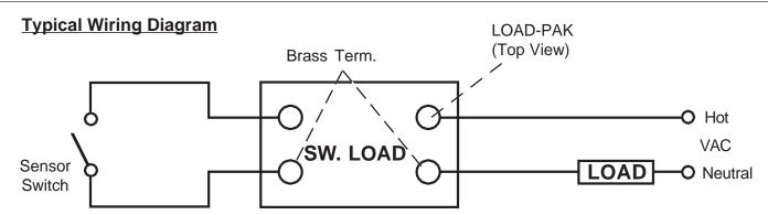
Wires connecting external sensor switches to LOAD-PAKS should not be placed in raceways or conduits containing high voltage lines. Voltages induced from these lines may trigger the low-power, solid-state triac; causing it to turn "on" momentarily.
